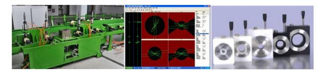
Uses the most advanced computer digital electronic technology and digital eddy current testing technology, can achieve high-speed data processing, and the detection rate can reach as high as 300M/ min. Automatically record and display the defects and their position, automatically generate inspection reports after detection (including the number of inspection, acceptance number and rejection number.)
